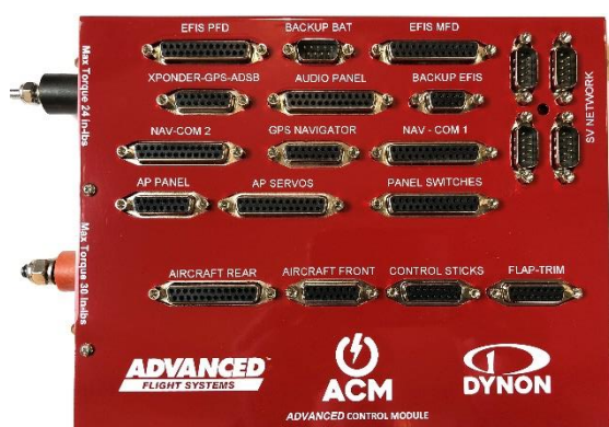
ACM module with Electronic Circuit Breakers
