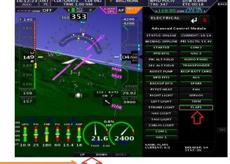
**10. Endpoint Slop Timeout** The Flap Motor will continue to run for this number of seconds to make sure the flaps are fully retracted or extended. The flap positioning system should not be used to provide an accurate position stop for full flap up or down settings.
