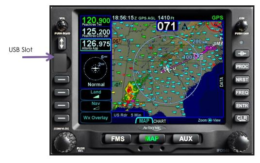
To enter configuration mode you will need to power up the IFD with a USB memory stick.
