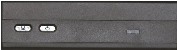
Figure 13 - D1 Top Side (left to right): Menu Button, Power Button
