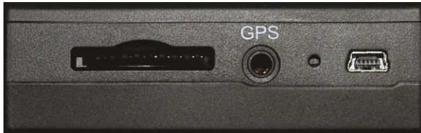
Figure 12 - D1 Left Side (left to right): SD Card , GPS, Reset, Mini-USB
