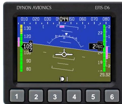
User interaction takes place via the EFIS-D6 main display and the six buttons beneath.
