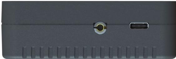
Figure 1 - D3 Left Side (left to right): GPS, USB-C
