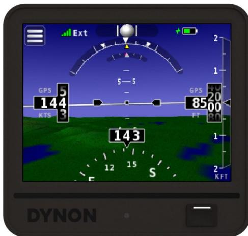
Figure 2 - D3 Front: Power Button (lower right)
