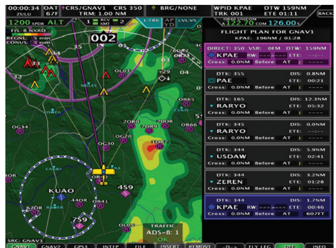
Flight Planning: Loads multi-leg flight plan from an external GPS navigator or allows user input from EFIS Screen.
