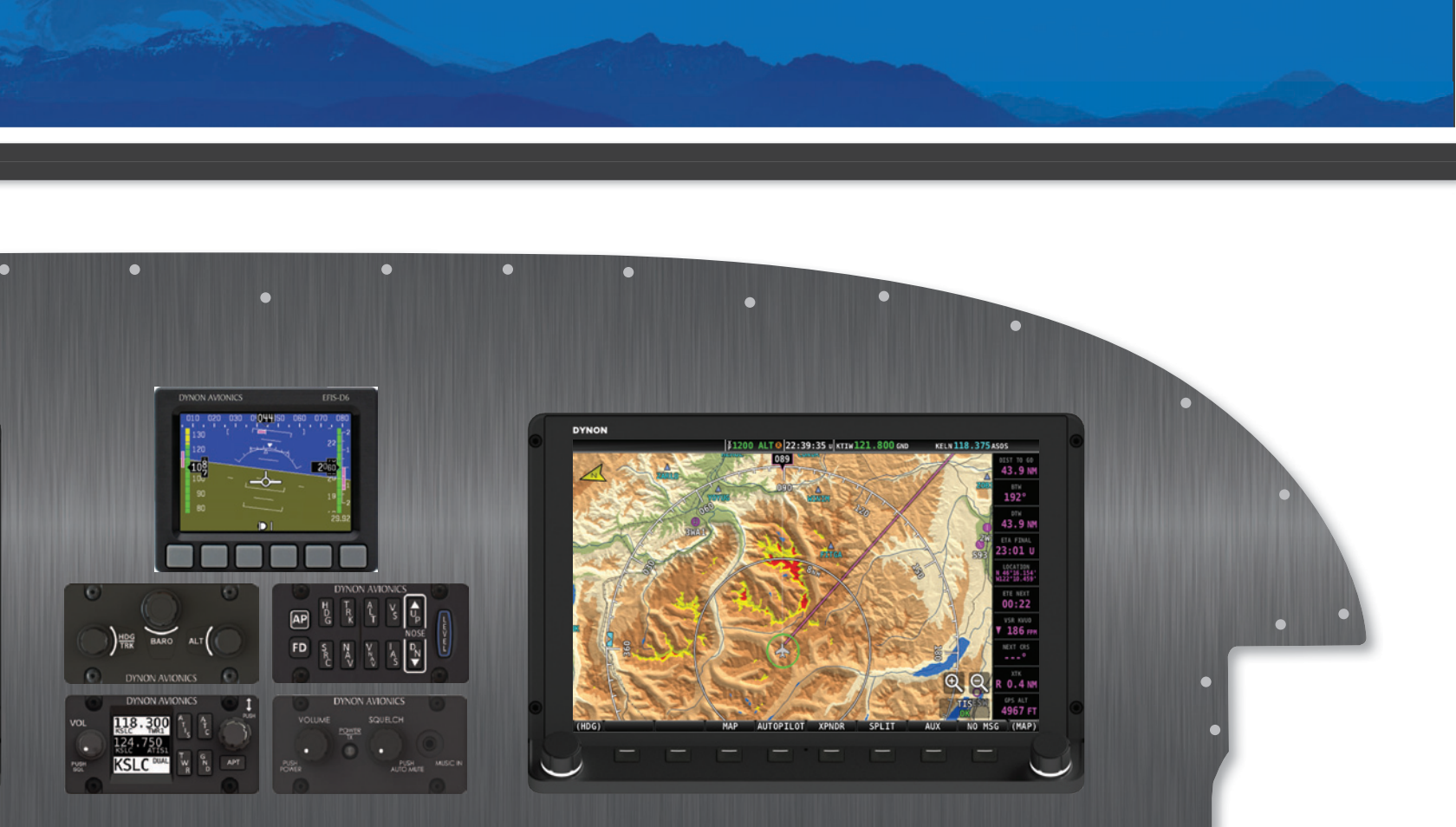
A Dynon EFIS-D6 offers an inexpensive independent backup set of flight instruments.
