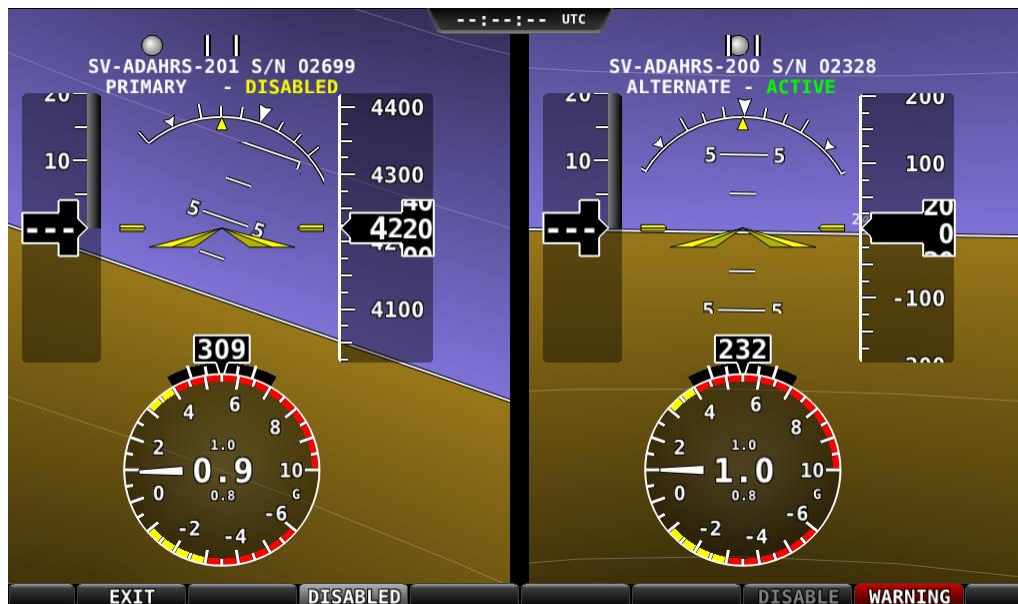
Figure 57 – ADAHRS Cross-Check Comparison (one ADAHRS disabled)
