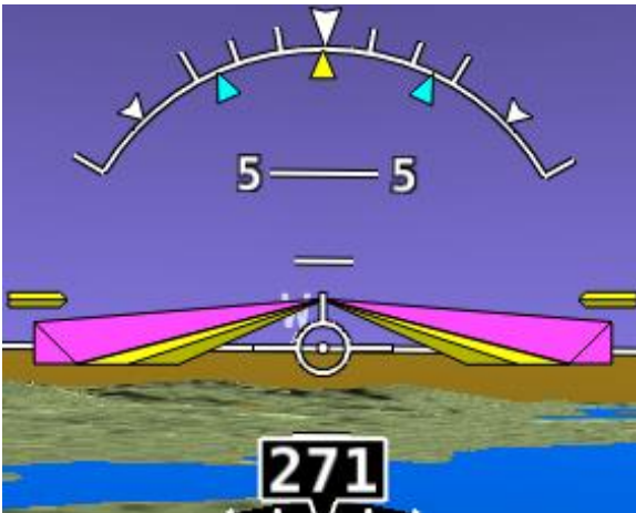
Figure 214 – Single Cue / Inverted-V with Autopilot Servos Engaged
