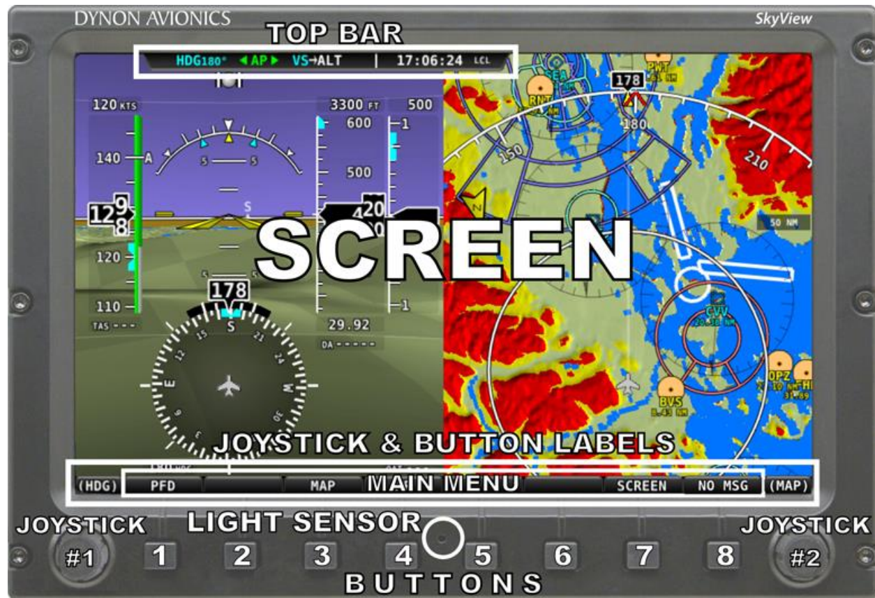
Figure 1 – SkyView Display Front Bezel Layout
