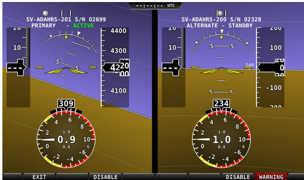
Figure 56 – ADAHRS Cross-Check Comparison
