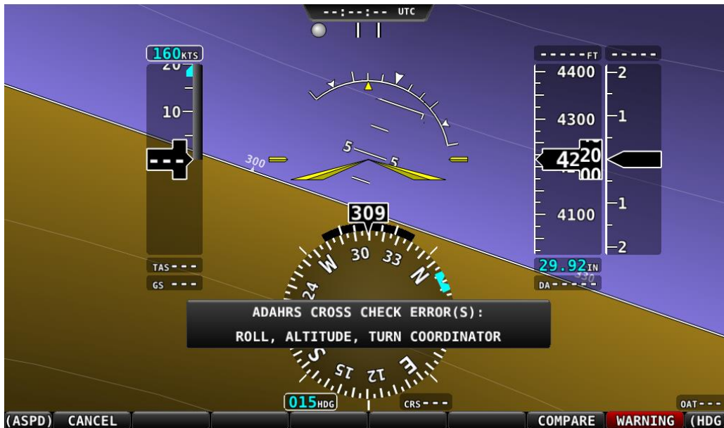
Figure 55 – ADAHRS Cross-Checking Disagreement
