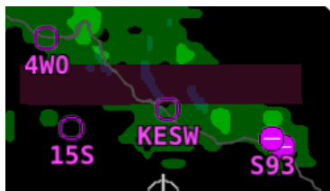
Figure 162 – Missing NEXAD Data Blocks
