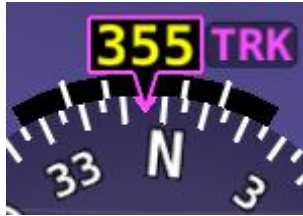
Figure 23 – GPS Track substitute for Magnetic Heading
