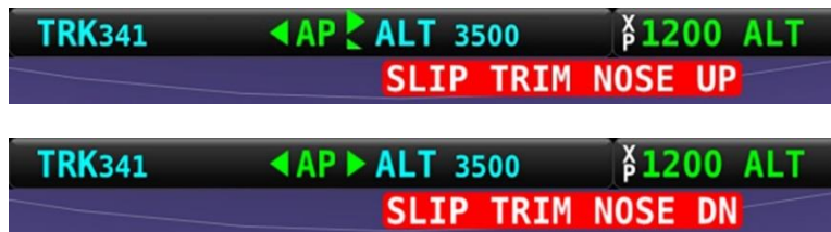
Figure 185 – Pitch Slip Trim Nose Up and Down Alerts
