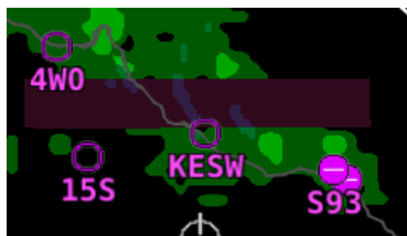
Figure 162 – Missing NEXAD Data Blocks
