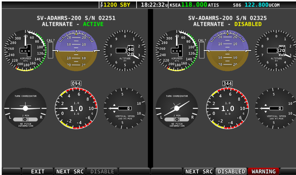
Figure 58 – ADAHRS Cross-Check Comparison – six-pack
