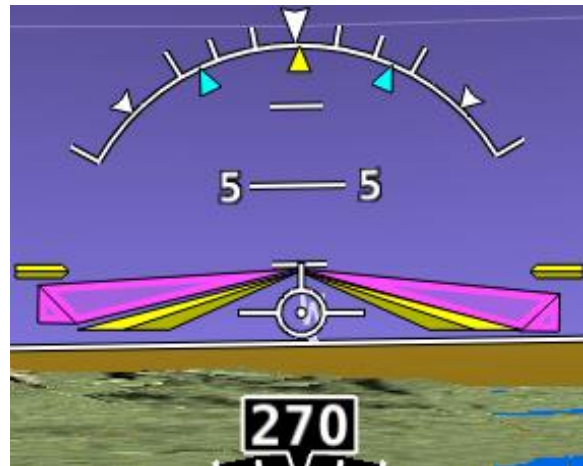
Figure 216 – Single Cue / Inverted-V with Autopilot Servos Not Engaged
