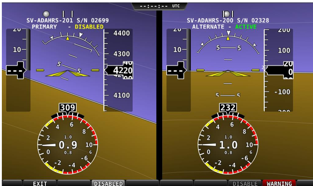
Figure 57 – ADAHRS Cross-Check Comparison (one ADAHRS disabled)
