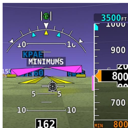
Figure 19 – MIN Bug and “MINIMUMS” Alert
