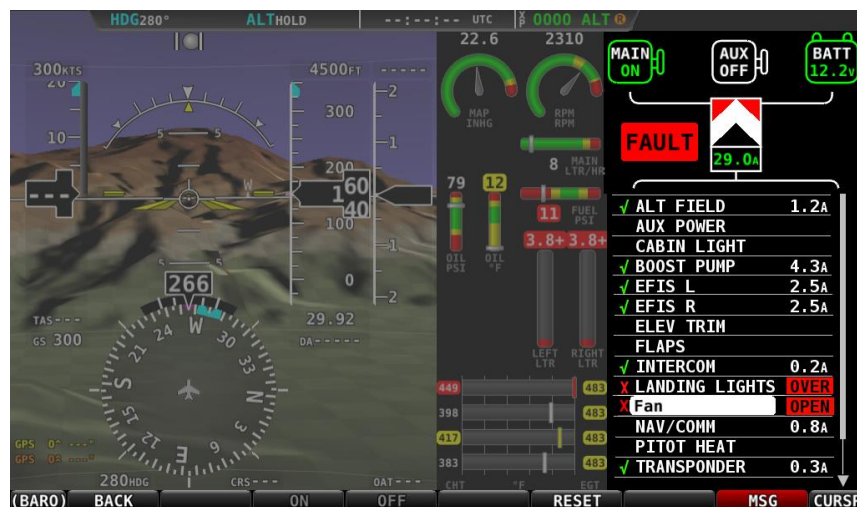
Figure 79 – VP-X Page with Fault
