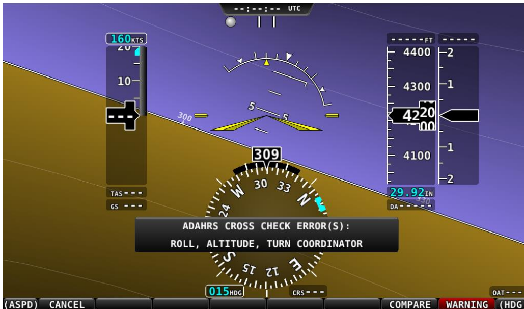
Figure 55 – ADAHRS Cross-Checking Disagreement
