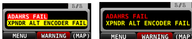
Figure 238 – Unacknowledged (left) and Acknowledged (right) Alarms
