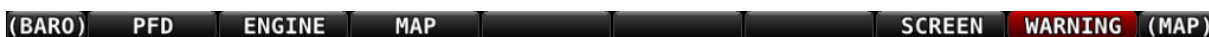
Figure 236 - Message Notification Area above button 8 (2nd from right), showing a Warning Notification
