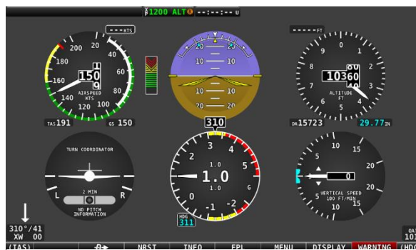
Figure 83 – G Meter in Six-Pack Presentation PFD
