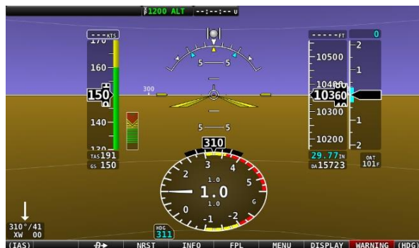
Figure 82 – G Meter in EFIS Presentation PFD
