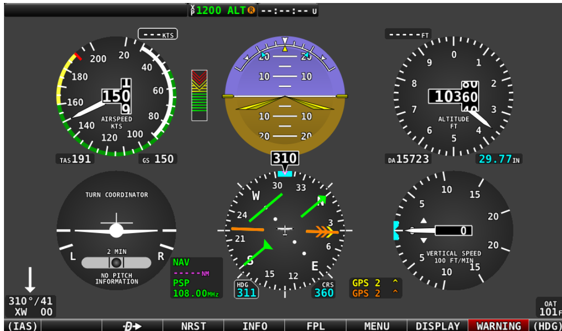
Figure 78 – Six Pack PFD Presentation, Synthetic Vision Disabled
