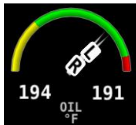
Figure 38 – Example of Combined Oil Temperature Widget Styles
