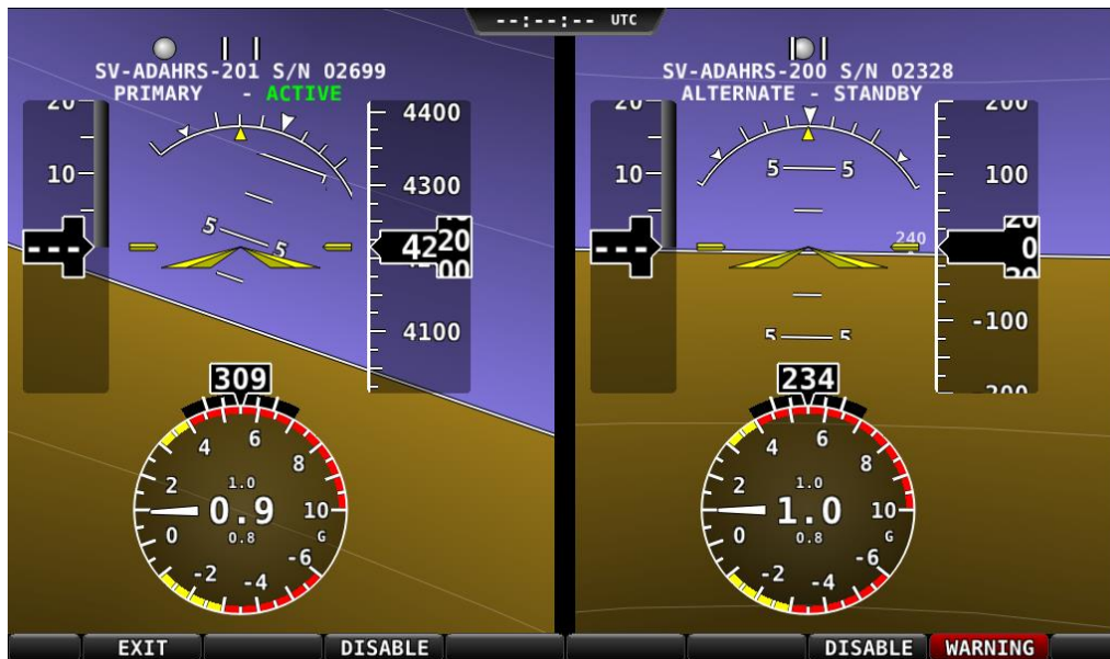
Figure 27 – ADAHRS Cross-Check Comparison
