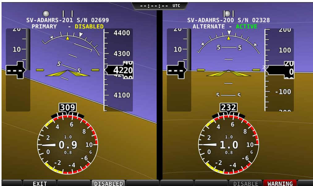
Figure 28 – ADAHRS Cross-Check Comparison (one ADAHRS disabled)
