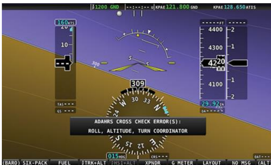
Figure 26 – ADAHRS Cross-Checking Disagreement
