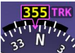
Figure 17 GPS Track substitute for Magnetic Heading
