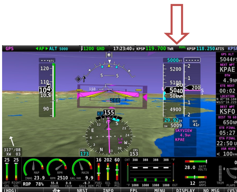
Figure 246: SkyView Top Bar Com Radio status overview
