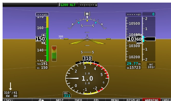
Figure 79: G Meter in EFIS Presentation
