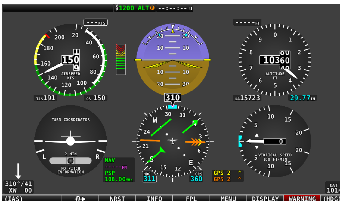
Figure 77: Six Pack PFD presentation, Synthetic Vision disabled.
