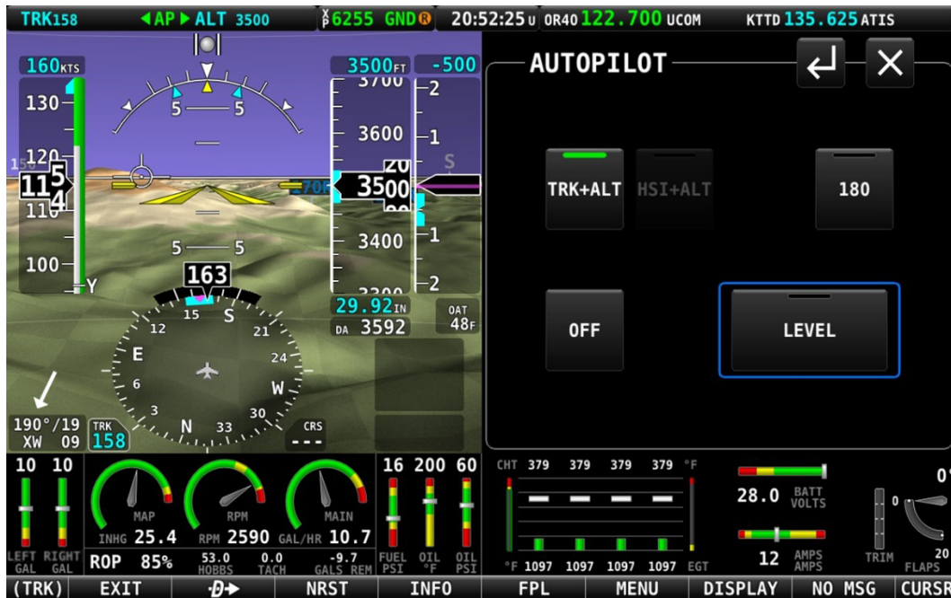
Figure 228: TRK+ALT mode is engaged.
