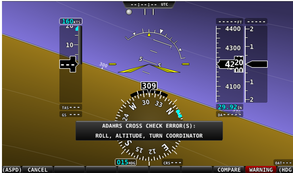
Figure 85: ADAHRS cross-checking disagreement.
