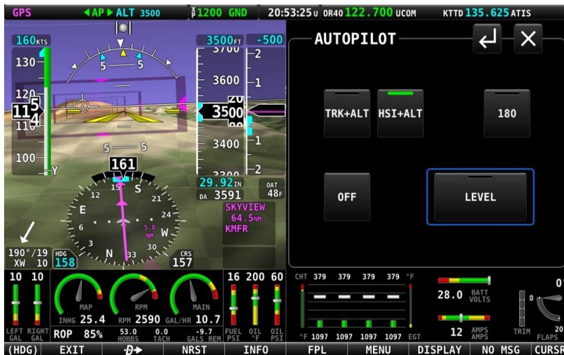
Figure 229: HSI+ALT Mode is engaged.
