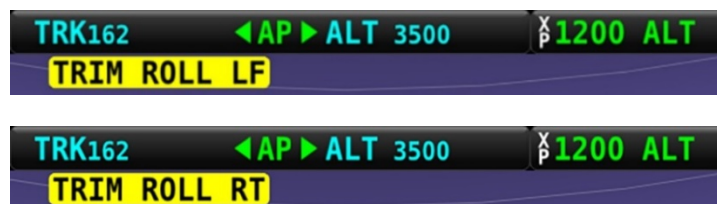
Figure 216: Roll Trim Left and Right alerts
