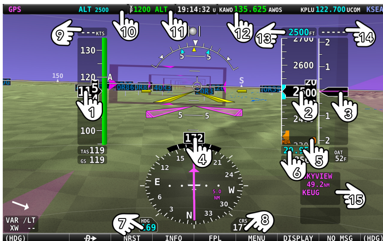
Figure 31: Touchable on-screen regions that change Knob BUG function.
