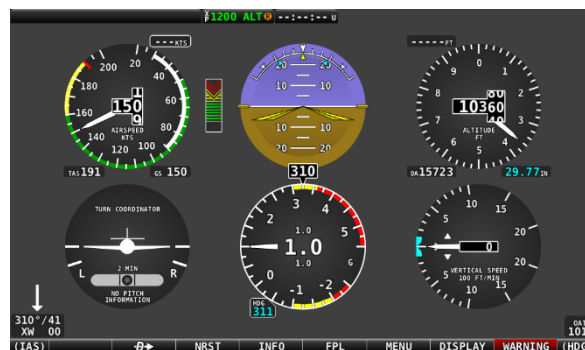
Figure 80: G Meter in Six-Pack Presentation
