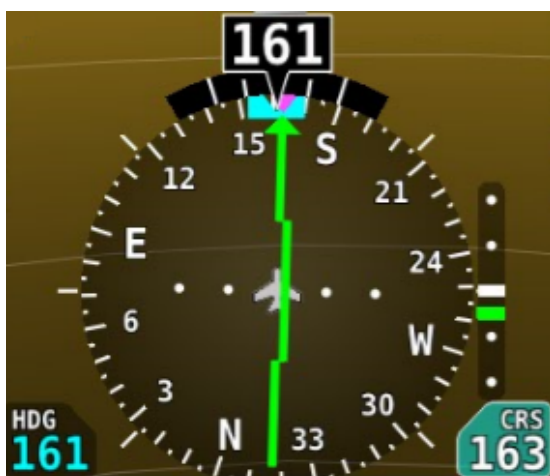
Figure 42: HSI example: Localizer
