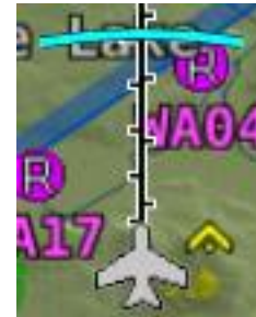
Figure 95: Altitude Intercept Arc
