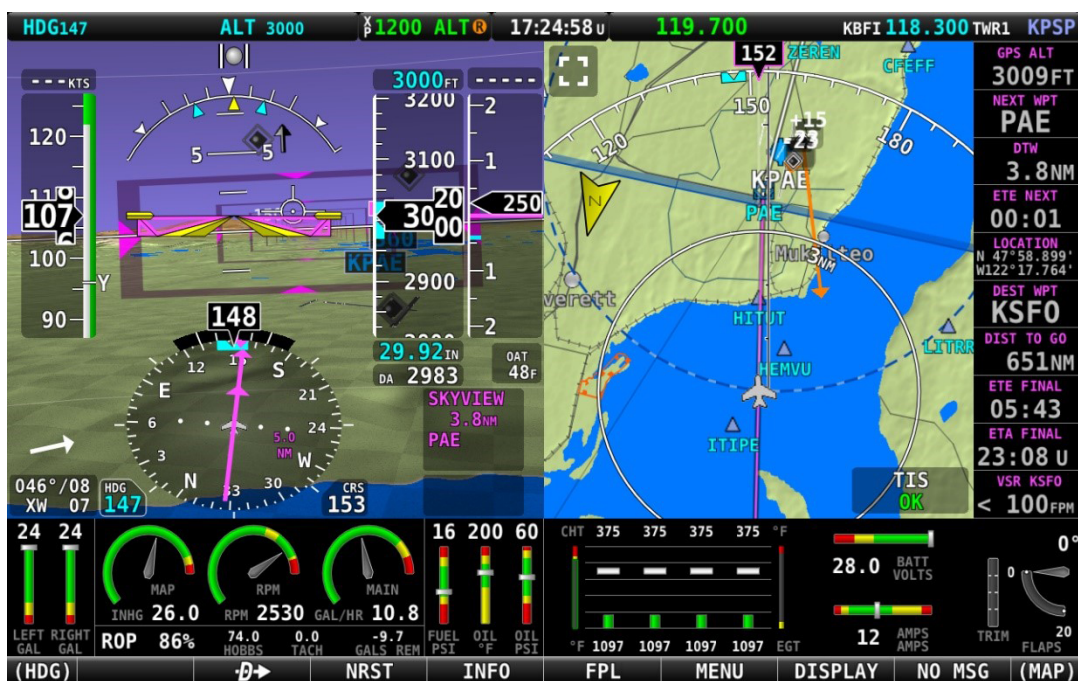
Figure 153: Active Flight Plan – HSI and MAP depictions
