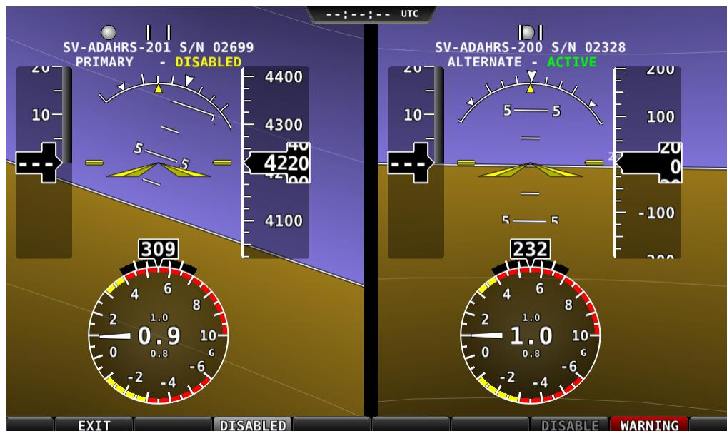
Figure 56 – ADAHRS Cross-Check Comparison (one ADAHRS disabled)
