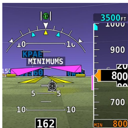
Figure 19 – MIN Bug and “MINIMUMS” Alert
