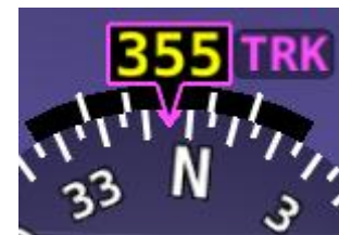
Figure 22 – GPS Track substitute for Magnetic Heading
