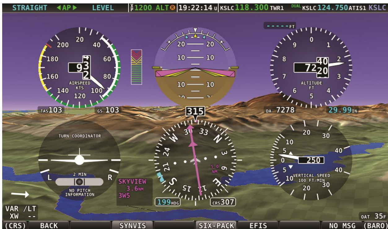
Figure 51 – Analog PFD with Synthetic Vision
