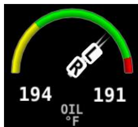
Figure 72 – Example of Combined Oil Temperature Widget Styles
