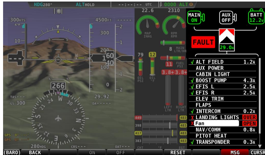
Figure 78 – VP-X Page with Fault
