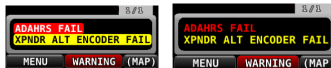
Figure 234 – Unacknowledged (left) and Acknowledged (right) Alarms
