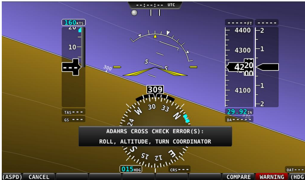
Figure 54 – ADAHRS Cross-Checking Disagreement
