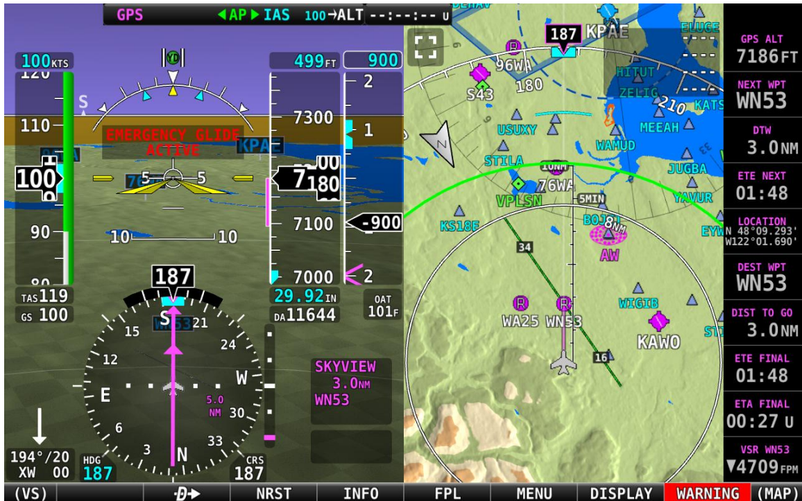
Figure 207: Emergency Glide Active alert
