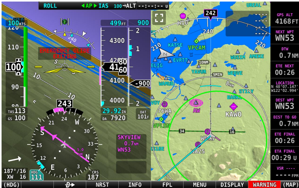
Figure 211: Emergency Glide Exiting alert
