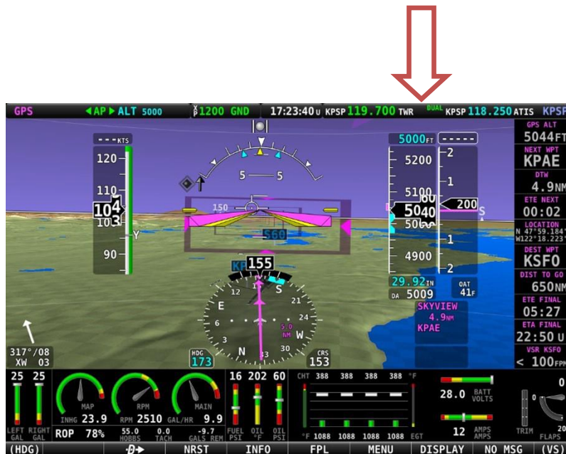
Figure 246: SkyView Top Bar Com Radio status overview
