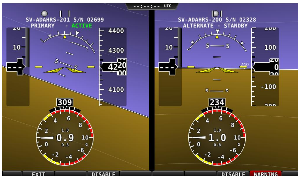
Figure 86 – ADAHRS Cross-Check Comparison (EFIS Presentation)
