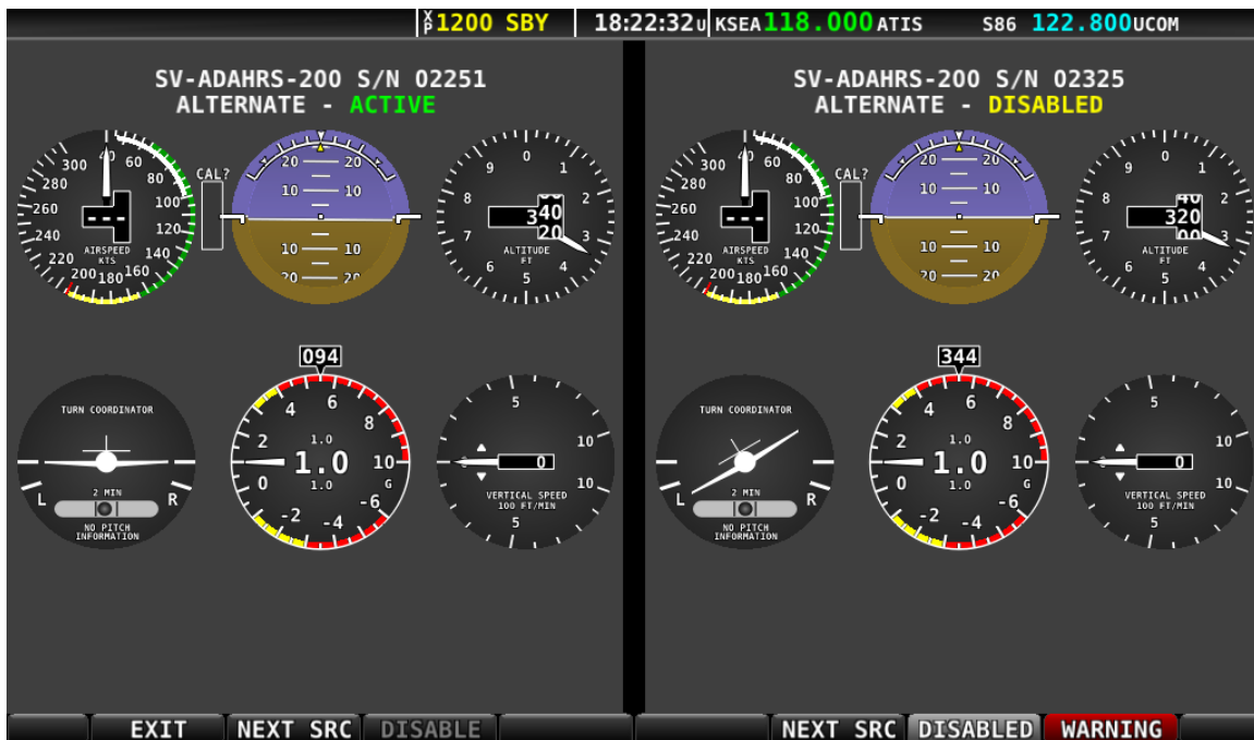
Figure 88: ADAHRS cross-check comparison (Six Pack presentation).
