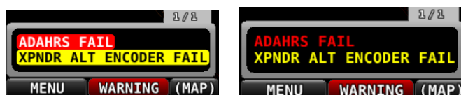
Figure 109 – Unacknowledged (left) and Acknowledged (right) Alarms
