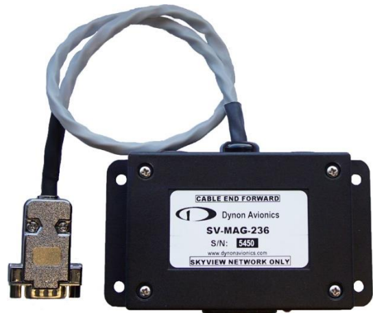
Figure 52 – SV-MAG-236 Remote Magnetometer
