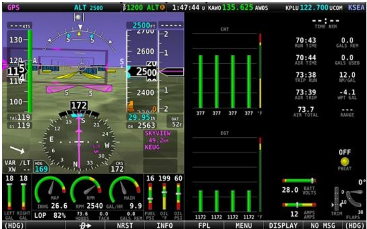
Figure 110 – 50% Page Layout with Engine Bottom Band Overwritten by 50% Page.
