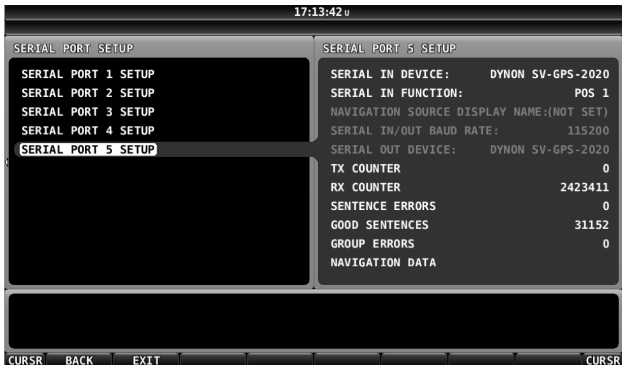
Figure 121 - Serial Port 5 Setup for SV-GPS-2020
