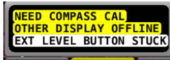
Figure 193 – EXT LEVEL BUTTON STUCK Message
