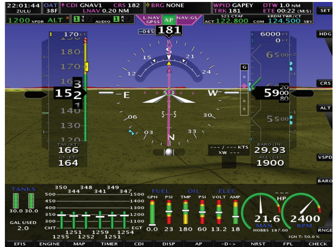
GPS and ILS Display: CDI and VDI displayed from external GPS navigator or Nav radio.
