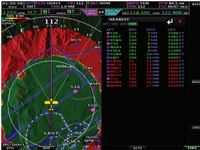
EMERGENCY Glide: Calculates and displays airports that are within your aircraft's engine-out glide range.
