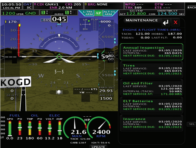
Aircraft Maintenance Logs: Keeps track and alerts you when it's time for Oil Changes, Annual Inspections, ELT Batteries, Filters, Brakes or any other user configurable item.
