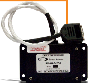
SV-MAG-236 Remote Magnetic Compass
