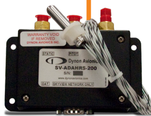
SV-ADAHRS-200 (Primary) Attitude & Pitot Static
