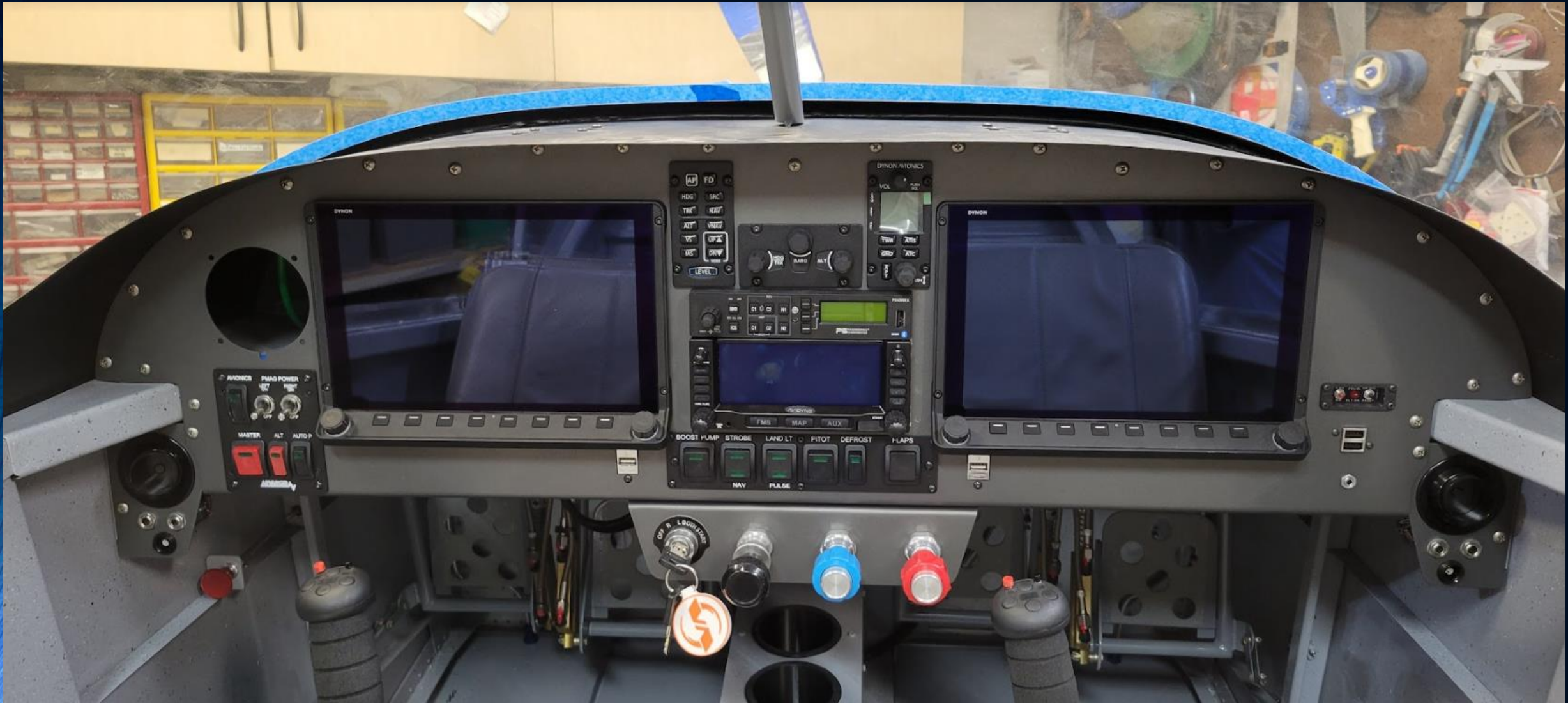
Panel Installation Van's RV-7
